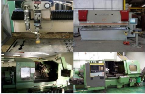
Our cnc lathes are capable of machining, drilling and threading a variety of parts from a variety of bar stock material (aluminum, steel, cast iron ) Anything ranging from 1/2" up to 10" Diameter.
